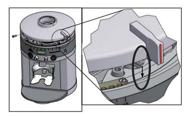
9.1.10 Carefully lay the grinder on its side. Reassemble the three screws under the base plate. Reposition the grinder on its rubber feet.
